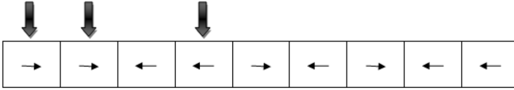
Fig. 1. Racetrack memory with multiple heads
